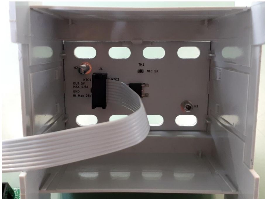
Inside view of upper part of enclosure with 5V regulation section
